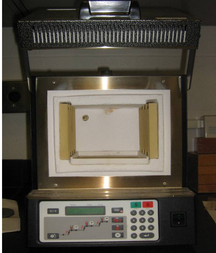
Figure 18. Vulcan Ceramic Furnace Oven Chamber. The oven door is hinged at the top which adds additional time to manipulate samples both into and out of the chamber. The furnace can be set to run at a steady state temperature or adjust the chamber temperature at regulated intervals.
