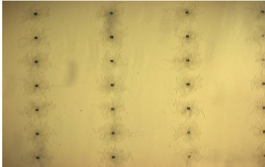
Figure 20. Successful Growth in Holes. This is the culmination of multiple attempts of both spore application and removal until a repeatable, reliable technique was developed. The center of gravity for the growth of B.t. on this etched slide is clearly the holes. The area between the columns is clear of excess surface spores.
