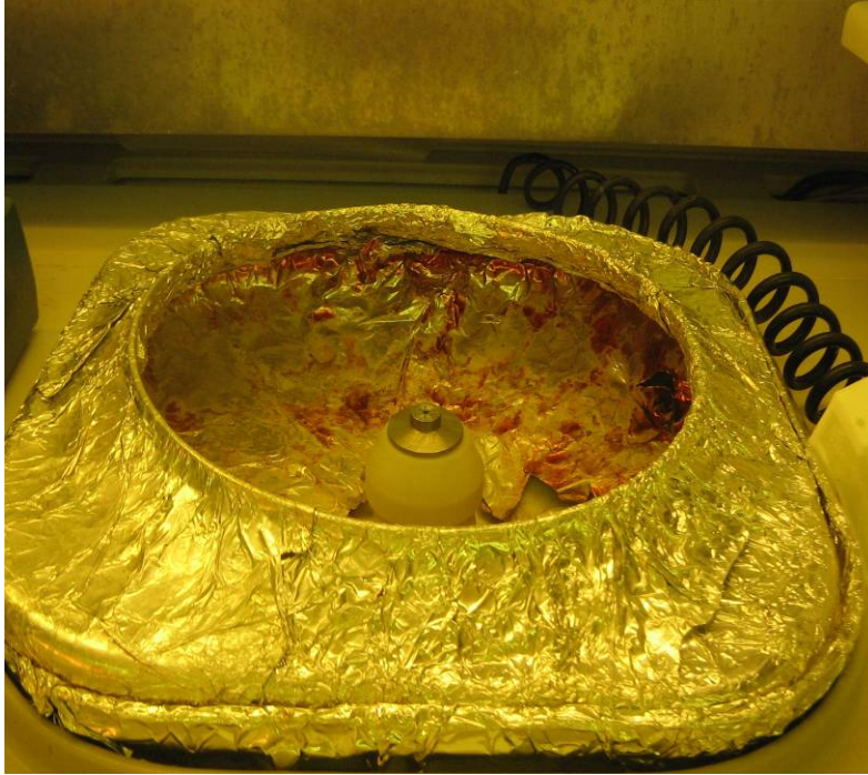
Figure 7. Solitec model 5100 Manual Single-head Spinner. The large vacuum chuck in the center holds the glass cover slip firmly in place while the chuck rotates at the selected RPM. The spinner well is covered in aluminum foil for ease of cleaning as excess photo resist is deliberately flung off the spinning surface by centripetal force. A small drain below the chuck allows excess photo resist to flow into a collection container for proper waste disposal.
