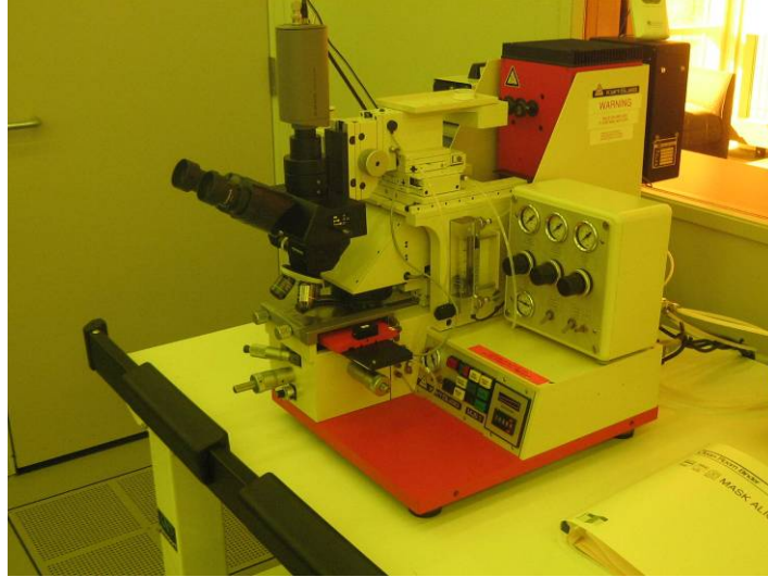
Figure 9. Karl Suss MEMS. The mask aligner has a movable stage where both the mask and the cover slip platform are inserted under the UV lamp. This stage is adjustable in both the horizontal and vertical directions. The eye piece and camera allows the user to manually align the mask and platform surface horizontally. In the vertical plane, it is critical for the mask to make mechanical contact with the photo resisted surface to prevent the UV light from damaging the area surrounding the mask windows.
